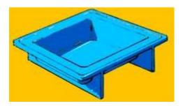
Production moulds are generally made from GRP and are manufactured to be rigid to maintain dimension stability. They are usually made from a timber pattern or plug.
